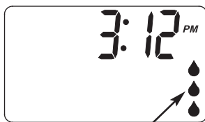
Droplets indicate water flow through conditioner
